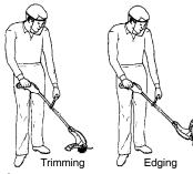
WARNING: Always wear eye protection. Never lean over the trimmer head. Rocks or debris can ricochet or be thrown into eyes and face and cause blindness or other serious injury.
